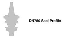
The Seal needs to be placed in a different position dependant on whether the Pipe is to be jointed with a socketed one or plain ended one.
